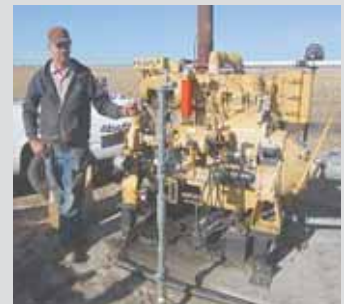
Norman Bredthauer converted his diesel irrigation engine to natural gas fuel and says he saves thousands of dollars a year on fuel costs.
