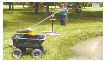
A broad pitchfork attaches to one end of a 21-ft. long pipe. Taylor grabs a 4-ft. long Pipe rides on a small metal roller mounted on a pedestal base. T-handle to push or pull the pipe, and also to rotate it from side to side.
