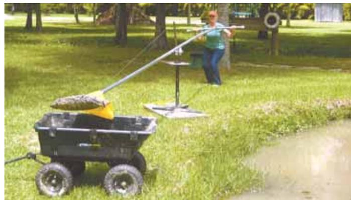
A broad pitchfork attaches to one end of a 21-ft. long pipe. Taylor grabs a 4-ft. long T-handle to push or pull the pipe, and also to rotate it from side to side.
