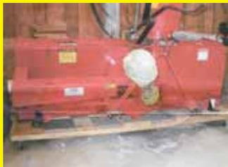
During the winter, I sometimes have to switch between my tractor's rear-mounted snowblower and my rear-mount winch for dragging downed timber. To make it easier to move them into position for mounting, I built wood frames on casters to roll them into place. The heavy-duty casters make them fairly easy to move around and hook up. Saves a lot of frustration when it's cold out. (Richard Diefenbach, Danville, Vt.)
