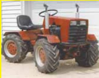
Not being able to buy a full-sized "toy" to play with, I decided to build a small one out of a pair of Case 220 garden tractors I already owned. I used one of the frames, cutting it at the center to articulate it. I then fitted the frame with both rear ends, hooked up the hydrostats to the drive motors on the wheels, and installed a 20 hp. Onan engine to power it. It looks and works great. (Ron Burt, 1776 Crouch Road, Jackson, Mich. 49201)
