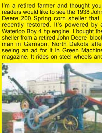
is designed to be belt-driven off a small tractor or gas engine. When on display it's shown with the Waterloo Boy engine.
