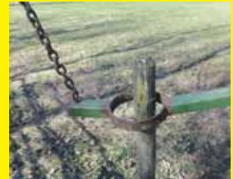
with about 1 ft. of sq. tubing welded to it on opposite sides. A length of chain is fastened onto both ends of the tubing so the tubing can be tipped with my front-end loader. Metal teeth welded on inside the pipe help it grip the post. I just drop the pipe over the post, tilt the loader bucket, and lift the post out. (Dave Marsh; brokefarm78@gmail.com)
