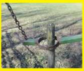
with about 1 ft. of sq. tubing welded to it on opposite sides. A length of chain is fastened onto both ends of the tubing so the tubing can be tipped with my front-end loader. Metal teeth welded on inside the pipe help it grip the post. I just drop the pipe over the post, tilt the loader bucket, and lift the post out. (Dave Marsh; brokefarm78@gmail.com)
