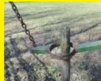
with about 1 ft. of sq. tubing welded to it on opposite sides. A length of chain is fastened onto both ends of the tubing so the tubing can be tipped with my front-end loader. Metal teeth welded on inside the pipe help it grip the post. I just drop the pipe over the post, tilt the loader bucket, and lift the post out. (Dave Marsh; brokefarm78@gmail.com)
