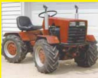
Not being able to buy a full-sized "toy" to play with, I decided to build a small one out of a pair of Case 220 garden tractors I already owned. I used one of the frames, cutting it at the center to articulate it. I then fitted the frame with both rear ends, hooked up the hydrostats to the drive motors on the wheels, and installed a 20 hp. Onan engine to power it. It looks and works great. (Ron Burt, 1776 Crouch Road, Jackson, Mich. 49201)
