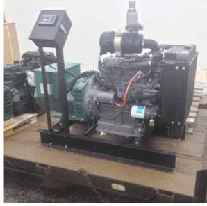
"Reefer" engines can be used to make lowcost gensets, savs Joas Bontrager, who pairs low hour Kubota engines with new generators.
