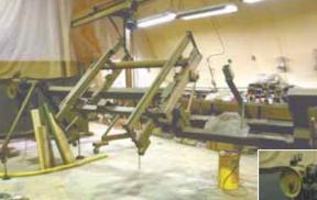
John Martens made this 360-degree welding table and hoist, which he uses to handle the frames on large liquid fertilizer caddies that he builds.
