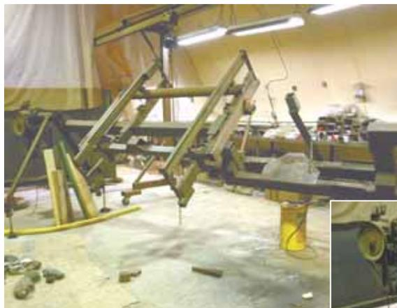
John Martens made this 360-degree welding table and hoist, which he uses to handle the frames on large liquid fertilizer caddies that he builds.
