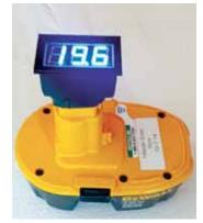
Digital battery tester attaches to the posts on any DeWalt 18-volt battery and shows the voltage in big, brightly lit numbers on top.
