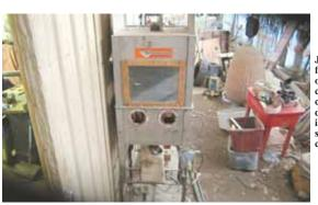
John Gass figured out how to convert an old commercial dishwasher into a sandblasting cabinet.
