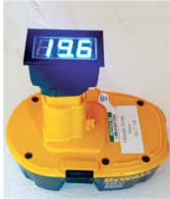
Digital battery tester attaches to the posts on any DeWalt 18-volt battery and shows the voltage in big, brightly lit numbers on top.
