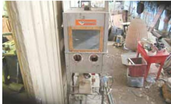
John Gass figured out how to convert an old commercial dishwasher into a sandblasting cabinet.
