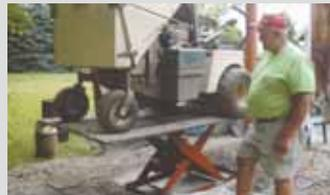
it for use as a service lift, which I use when working on my 3 Grasshopper riding mowers. The lift came with a 2 by 4-ft. top plate, and to make it big enough for the mowers I welded 39 in. of material on each end and 10 in. on each side. I used 1-in. sq. tubing to build a frame for the enlarged table and welded it onto the lift's original 2 by 4 base frame.
