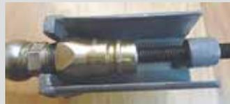
solved the problem by making a device out of a 3-in. C-clamp. I removed the swivel and drilled a depression in it so the tip of the coupler stays aligned. Then I welded iron onto the other end to hold the hose. A metal guard welded onto the clamp keeps any spraying oil away from me as I'm relieving the hose pressure.
