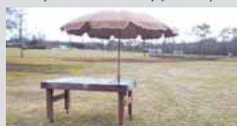
rides on four 4-in. caster wheels that I bought at Harbor Freight. I can easily roll the table around anywhere inside or outside the shop. I bored a hole into one end of the table so I can install a big umbrella when working outside. I use outlet strips with the shop's electrical outlets so I can hook up to 2 or 3 power tools at a time while I'm working at the table.
