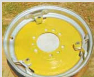
mounting tabs on the Farmall rim. I also enlarged the hole at center to fit the Farmall hub.
