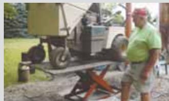
it for use as a service lift, which I use when working on my 3 Grasshopper riding mowers. The lift came with a 2 by 4-ft. top plate, and to make it big enough for the mowers I welded 39 in. of material on each end and 10 in. on each side. I used 1-in. sq. tubing to build a frame for the enlarged table and welded it onto the lift's original 2 by 4 base frame.
