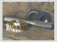
the application. We will test the hardness of the piece and decide on the best material for the purpose, take careful measurements, and reproduce a gear to those specifications. Heat treatment and finish grinding processes follow as needed," says Lapp.
