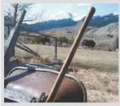
Paul Miller, Gardiner, Mont.: "A friend of mine ran over my wheelbarrow, breaking off one handle. I had an ax handle that was broken off at the head. I drilled holes in the ax handle, aligned it with the other handle, and screwed it onto the remaining broken off section. It is very comfortable to use. If I can find another ax handle, I'll ask my friend to run over the other side."
