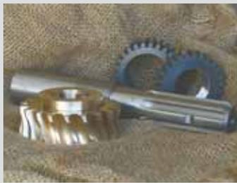
the application. We will test the hardness of the piece and decide on the best material for the purpose, take careful measurements, and reproduce a gear to those specifications. Heat treatment and finish grinding processes follow as needed," says Lapp.
