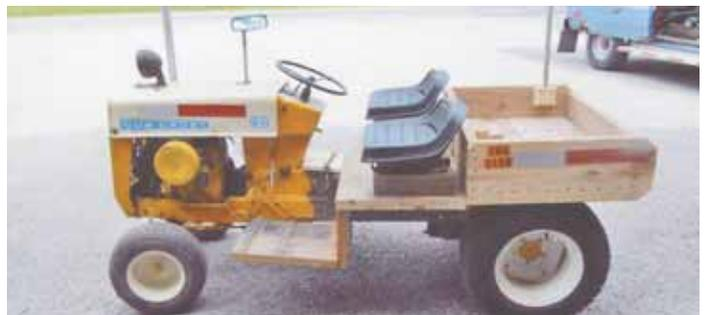
**Rollan Schnitker stretched out a late 1970's Cub Cadet garden tractor, added a 2-ft. long, 4-ft. wide wooden bed on back, and a second seat.**
