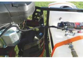
Sprayer is operated by a 12-volt pump that hooks up to mower's battery.
