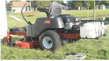
Fire ants are a real problem in Stan Bennett's area, so he mounted a quick-disconnect boom sprayer on back of his Toro zero-turn riding mower to control them.
