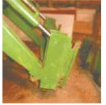
Bernard Schalgel used railroad rails to build this quick-tach mounting system for his tractor's front-end loader. "I can scoop up a bucket fast with no fear of structural failure," he says.
