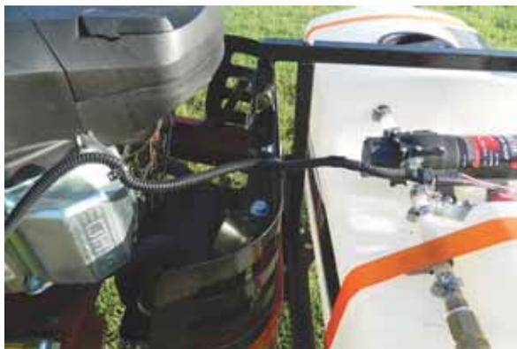
Sprayer is operated by a 12-volt pump that hooks up to mower's battery.
