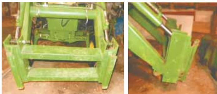
Bernard Schalgel used railroad rails to build this quick-tach mounting system for his tractor's front-end loader. "I can scoop up a bucket fast with no fear of structural failure," he says.
