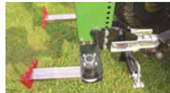
Edward Hollmen’s 2-wheeled log arch is equipped with a big claw on back and a pair of steel lift prongs up front, which together lift the entire log at the same time.
