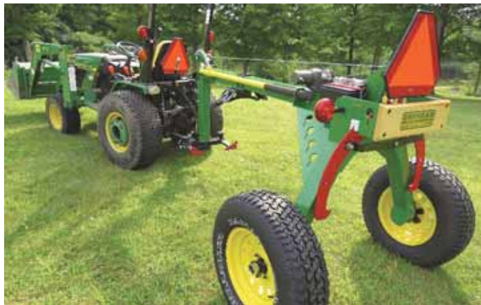
Edward Hollmen’s 2-wheeled log arch is equipped with a big claw on back and a pair of steel lift prongs up front, which together lift the entire log at the same time.
