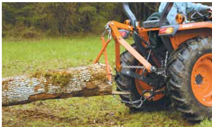
Tom Repko developed this 3-pt. mounted skidder to harvest firewood and thin Douglas fir trees on his 40 acres of timber. He now manufactures units for sale.
