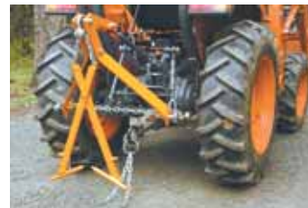
“The majority of the pulling load is from the tractor drawbar and below the rear axle,” says Repko.
