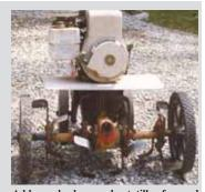
Add-on wheels propel rototiller forward and take all the work out of driving it around.
