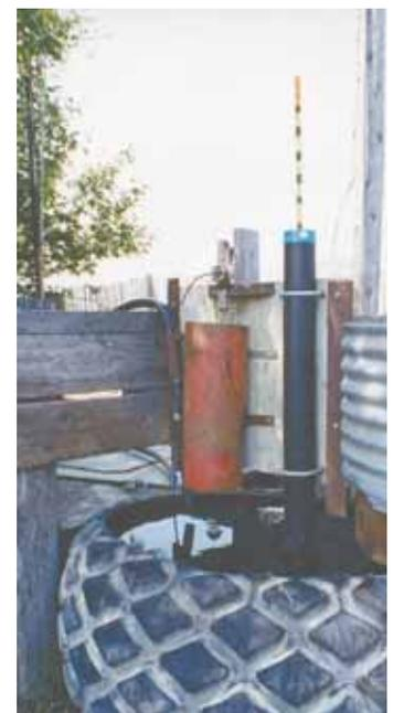
Float attaches to wooden dowel with orange cap on top. Yellow and black marks show exactly how full the tank is at all times.
