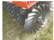
Their wavy coulters cut and mix residue while aerating the soil.
