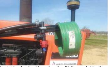
To protect the end nozzles on his spray boom, Darrell Snider screwed a 6-in. wide section of large dia., flexible pvc drainage pipe onto each end of the boom.
