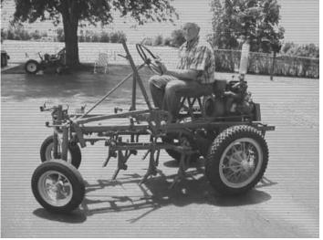
A number of Ford Model A parts, including the rear wheels and axle, were built into this homemade Allis-Chalmers tractor that's made to look like a model G.
