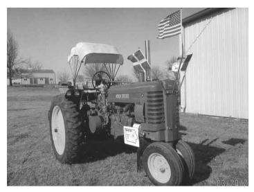
Maynard Hansen installed a starter with a matching flywheel and a Delco alternator on his 1941 Deere A, but that left him with a stopping problem. So he came up with a solenoid to go in the A's fuel line and tied it into his new electronics to shut it down.
