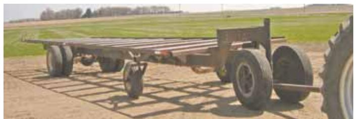
Bale wagon was converted from an old school bus and is fitted with a pedestal pivot on front (above). Wagon can carry 24 1,000-lb. bales at a time out of the field.
