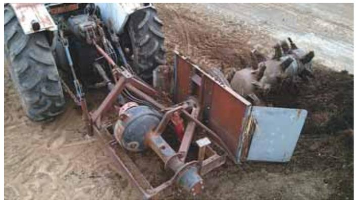
He built the 3-pt. mounted compost turner using a 20,000-lb. truck differential.
