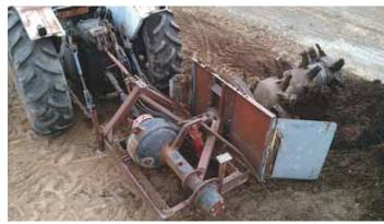
He built the 3-pt. mounted compost turner using a 20,000-lb. truck differential.
