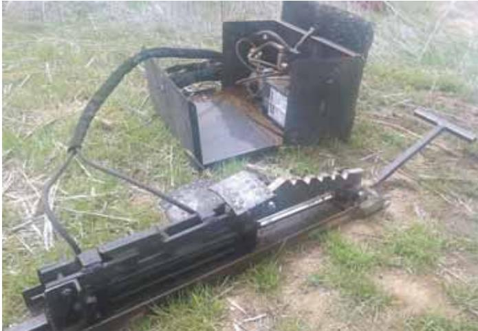
Terry Jacob uses his hydraulic culvert "reshaper" to fix damaged culvert ends that often plug up with heavy rains.
