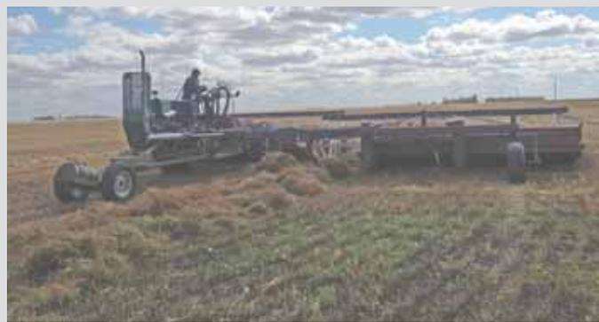
Back in 1977 **John Martens** used the engine, drivetrain and frame from an **Oliver 40** combine to build this twin-table swather. He says it's still working great.
