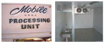
Knott's truck has hot water to wash down carcasses, a track to hang up to 3 cows or 40 pigs at a time, and a refrigeration system to cool the meat as he hauls it back to his processing facility.
