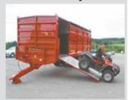
Trailer has a separate compartment up trailer drops down to serve as a ramp.
