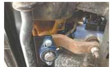
Tying the frame rails together and inserting the bearing eliminates flexing that causes steering to be slow or sluggish.
