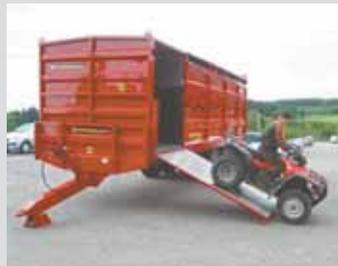
Trailer has a separate compartment up front to carry an ATV. A side section of trailer drops down to serve as a ramp.
