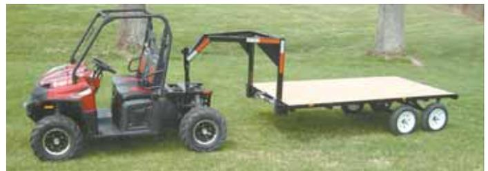
Tandem axle trailer is 5 1/2 ft. wide and 10 ft. long with a stake bed.
