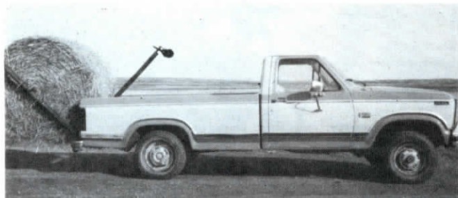
An angle iron hinge point chains to step bumper. To lift bale, a spear is pushed through center of bale by hand and chain loops on bale arms are slipped over spear ends.
