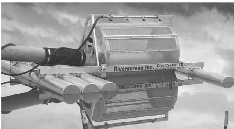
Water-driven, self-cleaning screen is designed to work in water as shallow as 4 in.
