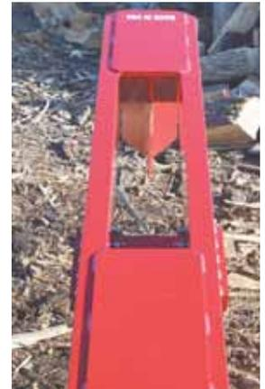
Log splitter is built from two pieces of channel iron mounted back to back, with an 8 by 24-in. "window" in between. The window design lets Trelstad see what he's doing and is also stronger than a single I-beam.
