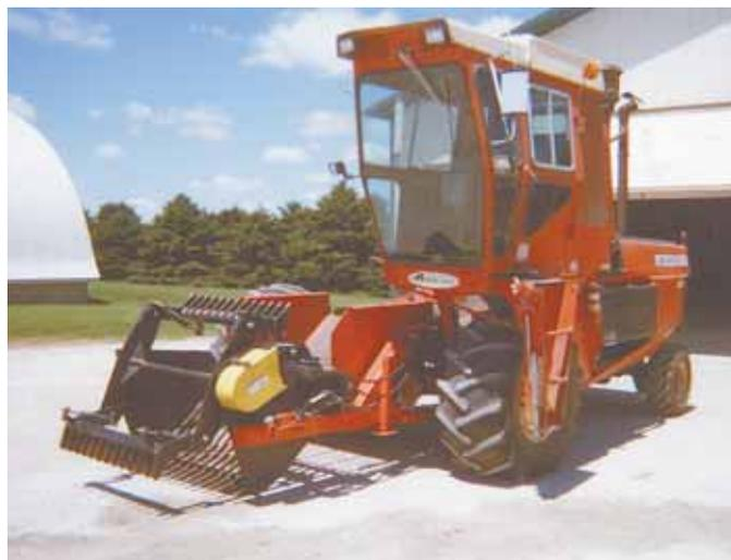
The 3 1/2-ft. wide, hydraulic-powered rock picker mounts in place of the Uni Harvester’s husking bed and corn head.
