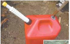
Brent Gill came up with his own vent for plastic fuel cans. "With the core valve removed, it's easy to fill a tank 3
