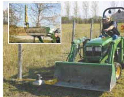
Hydraulic-powered cutter attaches to loader bucket.
