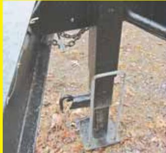
I was tired of reaching for the handle at the base of my trailer jack so I installed an extended handle to the base. I have a spring-loaded lock pin that I can pull out and turn it on the side, raise the base, and hit it with my foot to lock it in the up position. **(Larry Goodman, 3200 Welch Rd., Ionia, Mich. 48846 ph 616-755-1473)**
