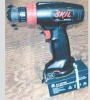
**Orley Killoran, Pincher Creek, Alberta:** "Here's how I salvaged my 12-volt cordless drill after the original battery packs failed. I bought a small 12-volt gel cell battery from a surplus store. Then I cut the top off an old battery case, extended the wires from the drill, and strapped the new battery onto the bottom.
