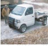
a rear bumper/hitch. I also converted the rear lights to LED's, added a headache rack equipped with lights, and undercoated the truck's frame and undercarriage with a Rhino-type bed spray.
