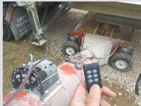
Remote-controlled Auger-Jogger makes it easy to move swing hopper into place under trucks and wagons.
