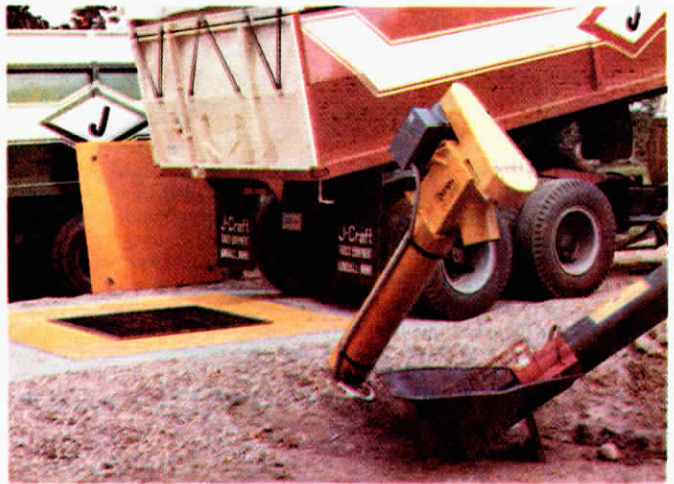
A stop/start switch automatically starts the auger as grain is dumped into the pit.
