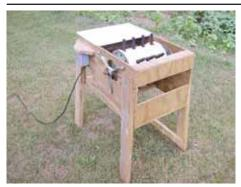
Jack McGee made this chicken plucker out of treated plywood, 12-in. pvc pipe, and parts from disassembled squirrel cage blowers.
