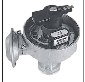
Electronic breakerless ignition system replaces points and condensers on old tractors.
