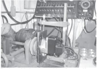
Photo shows a typical antique tractor magneto being tested on a commercial magneto bench tester.
