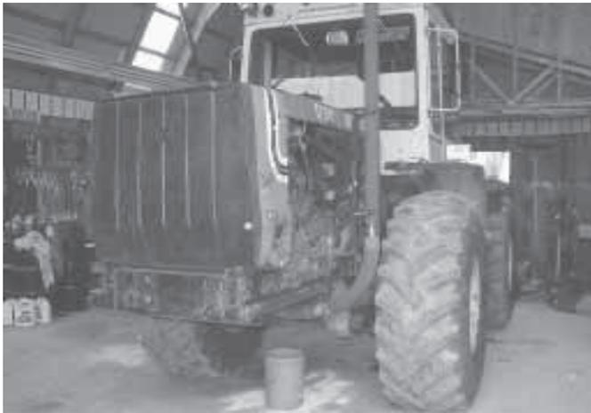
It took quite a bit of fabrication work, but Jim Ward was able to replace the engine in a Belarus 1790 4-WD tractor with a 466 DDT International.
