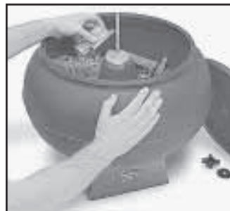
Eastwood jumbo parts tumbler uses vibration, not rotary action, to clean parts. It can hold parts up to 10 in. long.
