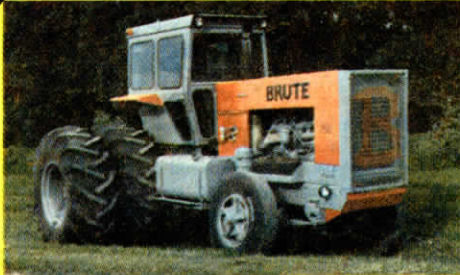
Going with two rather than four wheel drive simplified construction, says builder Stan Friesen.
