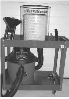
Air filter cleaner lets you use an air compressor to blow dust out of any canister-type filter.
