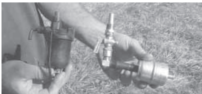
Adding tubing and an in-line filter can keep older tractor's fuel line from plugging up.
