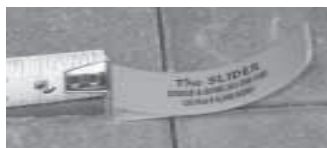
End of tape measure blade slips into a slot on the 3-in. Slider
