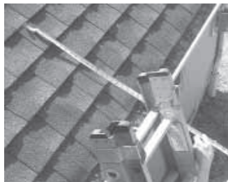
"Slider" allows free end of tape to slide smoothly over rough surfaces such as roofing.
