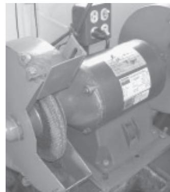
Bud Blanton stacked three chop saw wheels together and mounted them on his bench grinder. "Chop saw wheels cut at least twice as fast as grinding wheels," he says.
