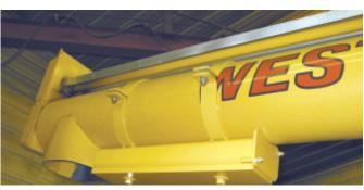
Gutschmidt added a weight box to counterbalance the lower end of his 10-in. by 36-ft. take-out auger, making it easier to lift (above). He attached a swivel caster wheel at the bottom to make the auger easier to roll ar ound.
