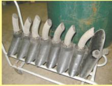
Roger Gutschmidt helped his church save on heating costs by "topping up" the building's existing insulation with Vermiculite. He drilled a series of holes in the walls and made funnels out of spray cones to blow the material in.
